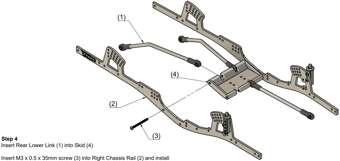
into rear hole of Skid (4) then loosely tighten screw
